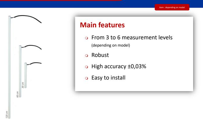
**HR Multi** is a multilevel soil moisture sensor. Low power consumption, reliable, easy to installusing an electric or thermal auger, and maintenance free, it has all the necessary assets to meet the expectations of meteorological services.
